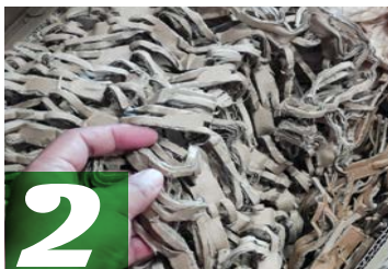
2 SHREDDING OF THE LEATHER SCRAPS INTO FIBERS
